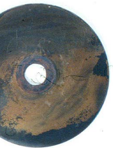
Fuji CrMoNiV steel DIN 30 CrMoNiV 5 11 (uncondensed steam)
