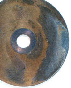
Fuji, 13% Cr stainless steel DIN X 20 Cr 13 (uncondensed steam)
